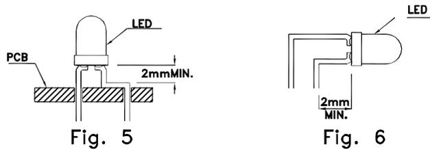
2. Lead forming or bending must be performed before soldering, never during or after Soldering.
